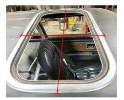
How to Measure a Sunroof: Measure OUTSIDE Frame where the edge of the sunroof touches the painted vehicle roof
