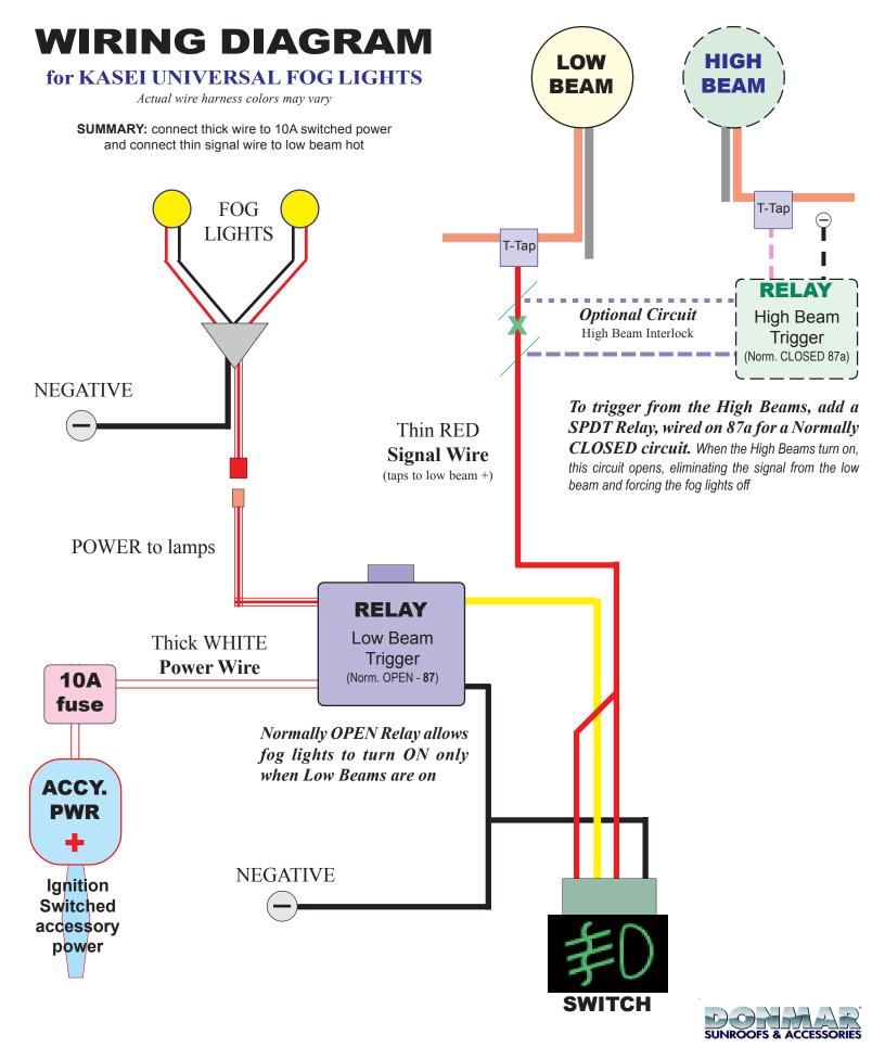
Universal Fog Light Harness only triggers off the <u>Low Beam</u>. If the vehicle low beams don't turn off when the high beams turn on, you can ADD another relay to turn off the fog lights.
