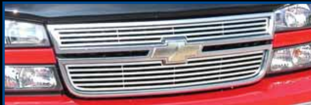
Stainless Steel Quarter by Quarter Style 2 Piece "Z" Grille 2006 Chevrolet Silverado 1500-3500 Pickup 2007 Chevrolet Silverado Classic 1003-0190-04
