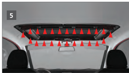
Bolting of the basic element (2) to the roof frame (1) with 24 pre-installed screws.
