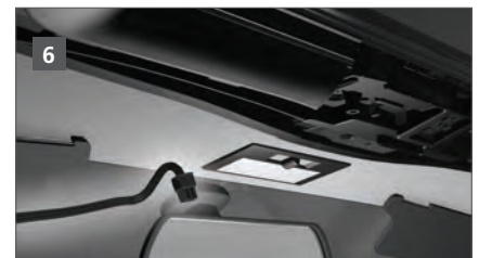
Insertion and connection of the spoiler roof's cable harness with the vehicle's electrical equipment (use of specific plugs is possible).
