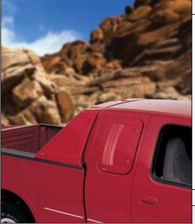
Lund Cab Fairings and Air Deflectors are an inexpensive and easy way to give your vehicle a sleek, highly-customized look while enhancing your driving experience. Cab fairings extend the lines of your truck's cab and provide protection from the sun. The Windjammer Air Deflector keeps your rear window cleaner and our Shadow Wiper Cowl protects your wipers.
